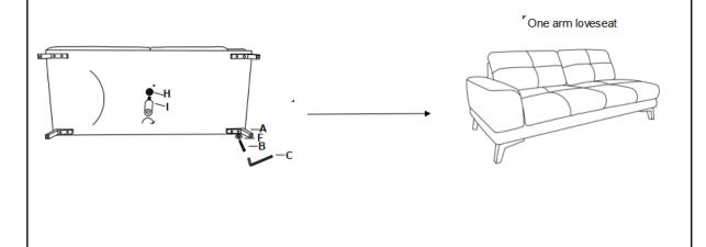
**STEP 2:**Attach Metal legs (A), bolts (B) and washers(F) with Allen key provided (C) and place in to each corner of the chaise. Attach plastic leg (I) and washer (H) in to the middle of the chaise turning to secure tightly.
